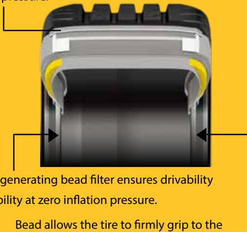
Low heat generating bead filter ensures drivability and durability at zero inflation pressure.
