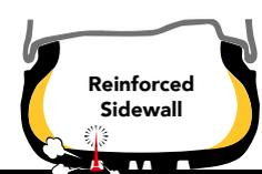
Temporary extended mobility for up to distance of 80km at speed of up to 80km/hr.
