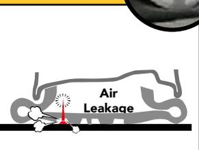
The pressure decreases immediately and the friction produces heat
