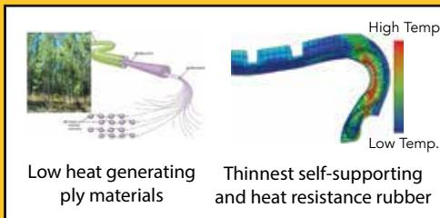
The optimal use of materials and components reduce the size of self-supporting rubber and reduce the stiffness of tire sidewall, improving riding comfort.
